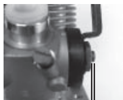
1/16" Low Speed Mixture: 1/16" of screw showing (1.5 mm) or 2 to 2 1/2 turns counter clockwise from clock.
